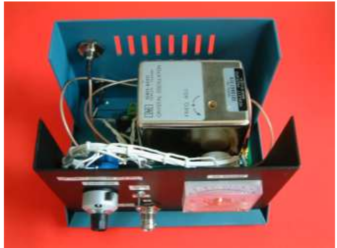
Figure 18. Interior View of OCVCXO and PLL
