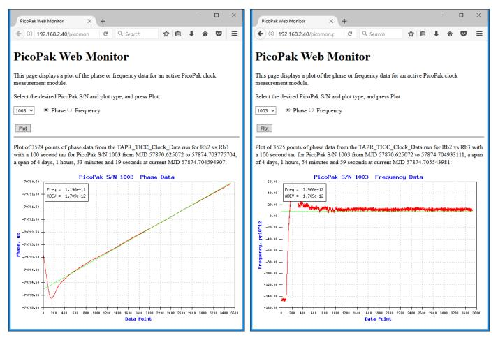
Figure 13. TAPR TICC Phase and Frequency Records Using PicoPak Database and Web Monitor
