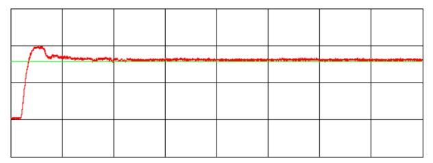
Figure 12. TAPR TICC Frequency Data Plot Using PicoPak Database and Monitor Program Vertical Scale=1x10<sup>-10</sup>/div, Horizontal Scale=12.22 hours/div Measurement Tau=100 s, Record Duration≈4 days, 2 hours
