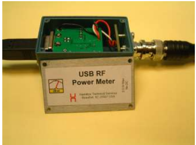
Figure 10. Assembled USB RF Power Meter
