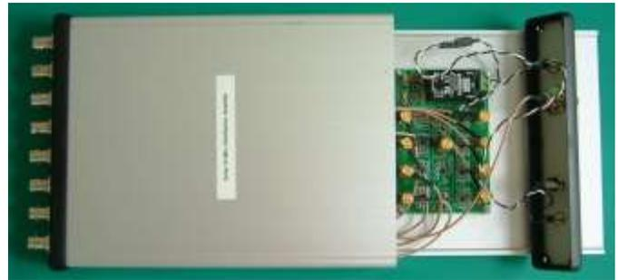
Figure 15. Interior View of Distribution Amp
