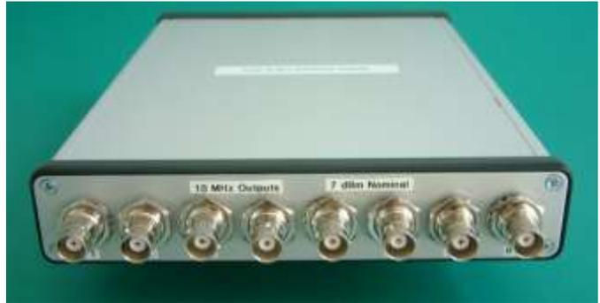
Figure 1. Octal 10 MHz Distribution Amplifier
