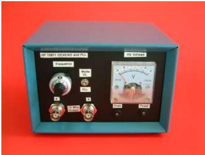
Figure 1. Photograph of HP 10811 PLL Module
