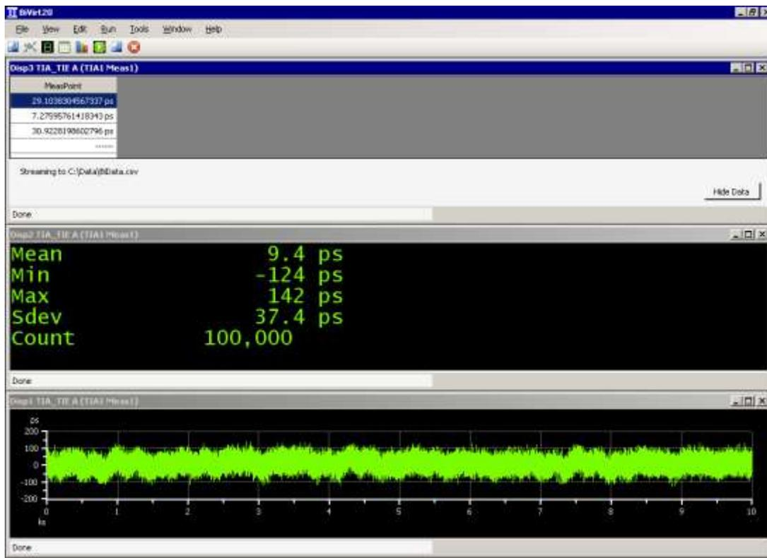
Figure 7. BiVirt Screen for 100,000-Point 0.1 Second Coherent Noise Test
