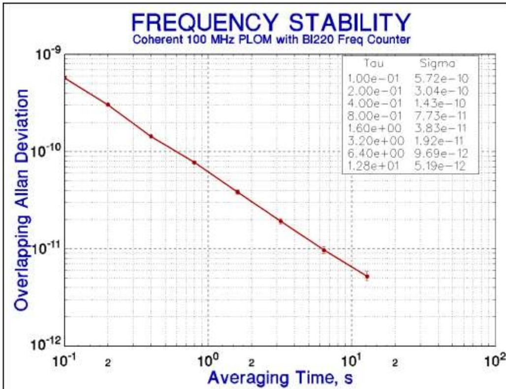
Figure 3. Frequency Stability – White PM Instrument Noise Floor
