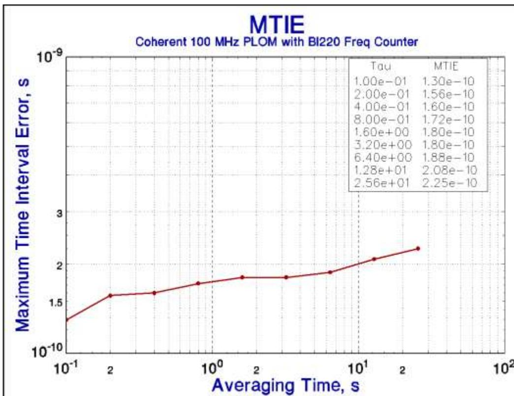
Figure 4. MTIE of Integrated Frequency Data
