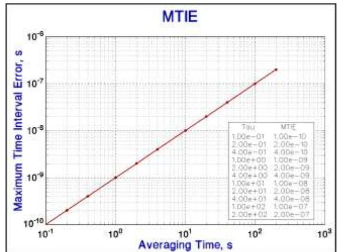
Figure 2.  $1 \times 10^{-9}$  Frequency Offset
